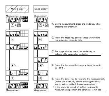
\* When the indication blank function is ON, the main display and sub display (Multi-display only) will be completely turned off. To turn them on, follow the steps above from step 1. (During parameter setup, the display blank function is turned off and the indication is turn on.) OFF(bright)  $\rightarrow$  B-3  $\rightarrow$  B-2  $\rightarrow$  B-1 (dark)  $\rightarrow$  ON (turn off)
