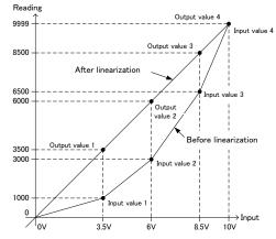
Setting for correction of the top figure Number of correction data : N-04
