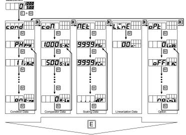
Press the Enter key to saves the data and returns to measurement mode. (Data are backed up with EEPROM even when the power is turned off.)
