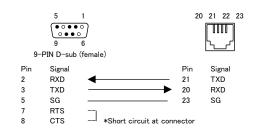
\* The host side CTS and RTS terminals connection is a typical example of a connection for hardware control. Please check with the system designer for details before making the connection.
