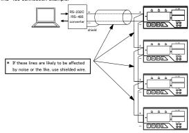
\* To enable the termination resistor, short-circuit terminals 21 and 22
