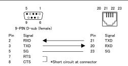
\* The host side CTS and RTS terminals connection is a typical example of a connection for hardware control. Please check with the system designer for details before making the connection.
