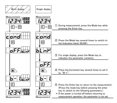
\* When the indication blank function is ON, the main display and sub display (Multi-display only) will be completely turned off. To turn them on, follow the steps above from step 1. (During parameter setup, the display blank function is turned off and the indication is turn on.) OFF(bright)  $\rightarrow$  B-3  $\rightarrow$  B-2  $\rightarrow$  B-1 (dark)  $\rightarrow$  ON (turn off)
