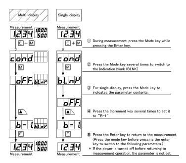
\* When the indication blank function is ON, the main display and sub display (Multi-display only) will be completely turned off. To turn them on, follow the steps above from step  $(D, (During parameter setup, the display blank function is turned off and the indication is turn on.) OFF(bright) <math>\rightarrow B-3 \rightarrow B-2 \rightarrow B-1$  (dark)  $\rightarrow ON$  (turn off)
