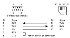
\* The host side CTS and RTS terminals connection is a typical example of a connection for hardware control. Please check with the system designer for details before making the connection.
