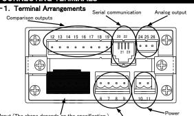
Input (The shape depends on the specification.) External controls
