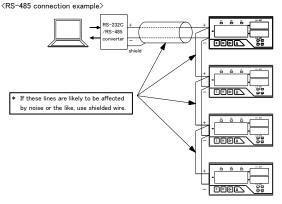
\* To enable the termination resistor, short-circuit terminals 21 and 22.
