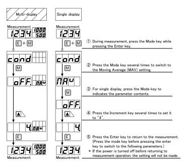
This function allows you to obtain a filtering effect without slowing down the sampling rate.
