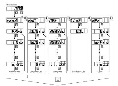
Press the Enter key to saves the data and returns to measurement mode. (Data are backed up with  $\ensuremath{\mathsf{EEPROM}}$  even when the power is turned off.)
