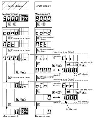
\* If the input actual value is out of range (OL), "Err" will be indicated and the original value will revert after 2 seconds
