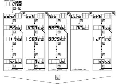
Press the Enter key to saves the data and returns to measurement mode. (Data are backed up with  $\ensuremath{\mathsf{EEPROM}}$  even when the power is turned off.)
